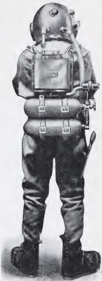
FIG. 50A.—SELF-CONTAINED DIVING DRESS. (SIEBE, GORMAN & Co.)
